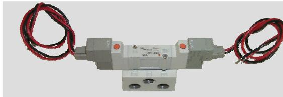
FESTO has also supplied two single solenoid valves. In order to wire the valves you must remove the white plastic pin protector that comes over the pins. Instructions in the package explain how to wire the valve. The fittings are the push to connect type so all you have to do is push in the tubing. The blue manual-override switch closes the valve for testing, but is spring-loaded and will not maintain the valve's position when released.
