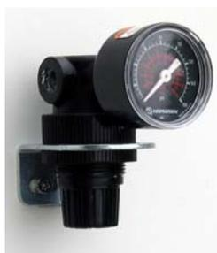
**Monnier** has donated the secondary regulator, which has a yellow ring around it. This is also a relieving regulator. Its purpose is to allow you to have a reduced pressure leg, if needed. There is an arrow denoting the direction of flow. The gauge may be placed in either of the other ports. The Monnier bag provides you with plugs to put into the gauge ports.
