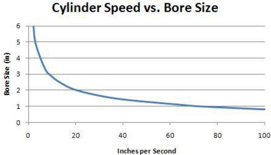
If the cylinder needed (based on force) will move too fast, then it can be slowed down by a special adjustable flow control fitting that screws into the cylinder ports. These fittings slow the air flow in one direction, so if only one is used a cylinder will be fast in one direction, but slow in the other. Using flow control on both cylinder ports will slow it in both directions.
