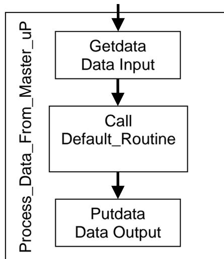
This structure ensures that 1) new inputs (joysticks, etc.) are continuously read in, and 2) the outputs (motors, Victors, Spikes, Solenoids, etc.) continuously receive new commands.
