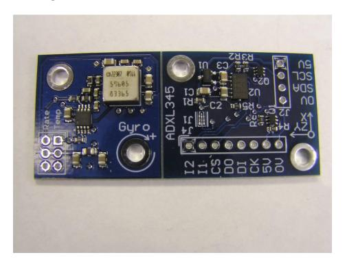
The sensor board in the 2011 FRC Kit of Parts hosts both an Analog Devices ADXL345 3-axis Digital Accelerometer and an Analog Devices ADW22307 1-axis Analog Gyroscope.
