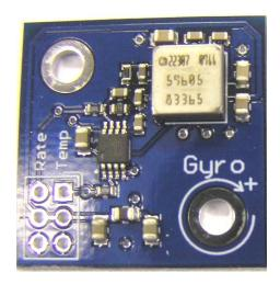
The angular rate sensor (gyroscope) senses angular changes about the top surface axis of the device and provides an output voltage proportional to the angular rate change. The output is useful for guidance, stability, and control of the robot platform. The lowest apparent drift on the gyro will occur when the module is mounted flat in or near the center axis of the robots rotation.
