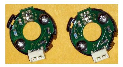
The US Digital E4Ps are incremental encoders outputting a 2-channel quadrature signal. They are capable of measuring shaft position, speed and direction, and fit on a 0.25" shaft. The encoders provided are 360 Codes per Revolution (CPR). With 4X quadrature decoding, you get 1,440 positions per revolution, which gives you a unique position every 0.25 degrees. The maximum RPM for these encoders is 10,000 RPM.
