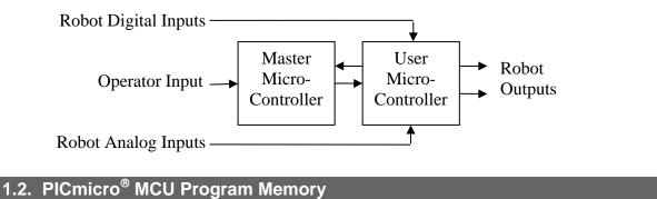
The PICmicro<sup>®</sup> in each Robot Controller has onboard FLASH memory that can be used to store the user's custom programs. This memory is non-volatile; meaning that it keeps its memory after power has been removed. There is a total of 32k bytes of memory space available to the user in which to store custom programs.
