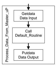
This structure ensures that 1) new inputs (joysticks, etc.) are continuously read in, and 2) the outputs (motors, Victors, Spikes, Solenoids, etc.) continuously receive new commands.
