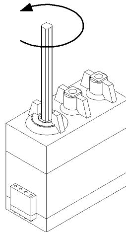
Example (using the default software): Press the Trigger button on the Port 1 Joystick to make a motor connected to RLY1 rotates clockwise. Press the Top button on the Port 1 Joystick to make a motor connected to RLY1 rotates counter-clockwise.
