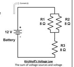
The sum of voltage sources and voltage drops in a circuit must equal zero
