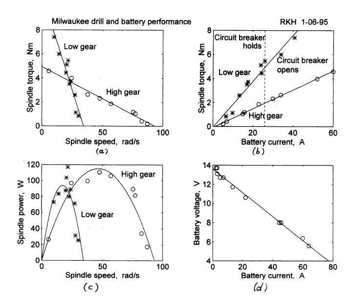
Figure 4.11: Performance curves for one drill motor with its gearbox, powered by one battery through a speed controller. (a) Torque vs. speed, (b) Torque vs. current, (c) Output power vs. speed, (d) Battery voltage vs. battery current.
