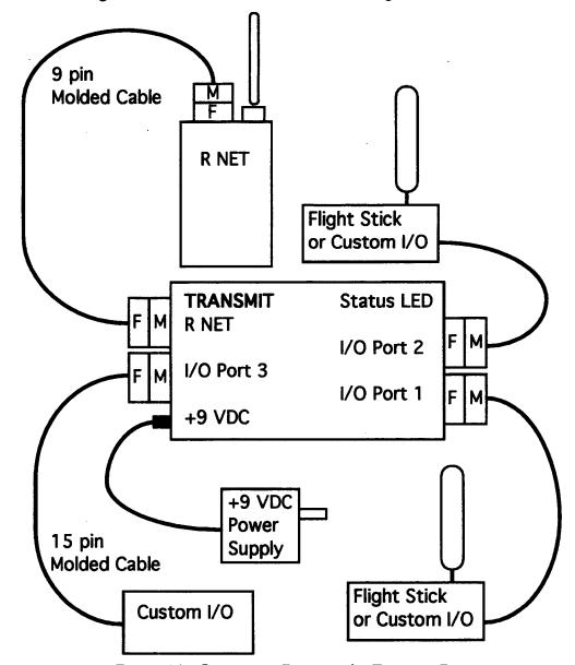
Figure 4.2 - Connection Diagram for Transmit Box
