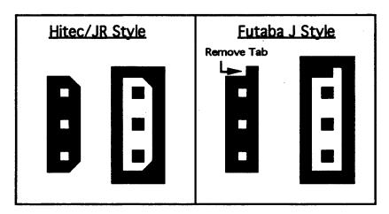
Figure 4.8: Hitec and Futaba-Style PWM Connectors
