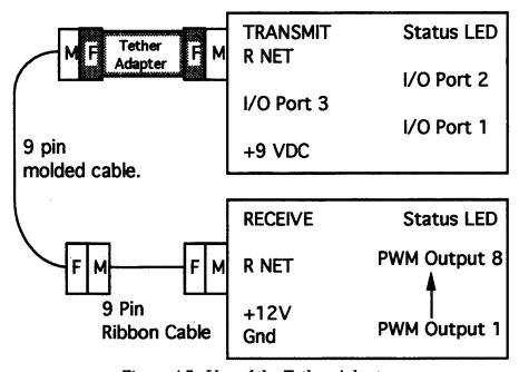
Figure 4.5: Use of the Tether Adapter
