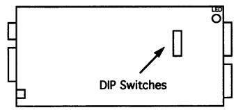
Figure 4.3: Location of DIP Switches Inside Transmit Box
