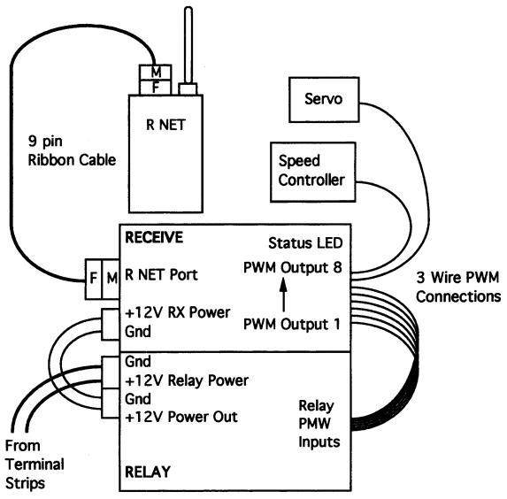
Figure 4.4: Receive/Relay Box Connections
