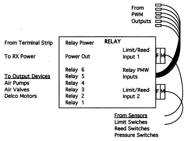
Figure 4.6: Relay board connections
