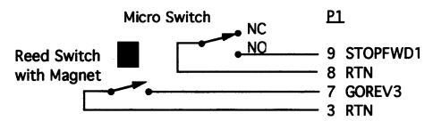
Figure 4.7: Example sensor wiring.
